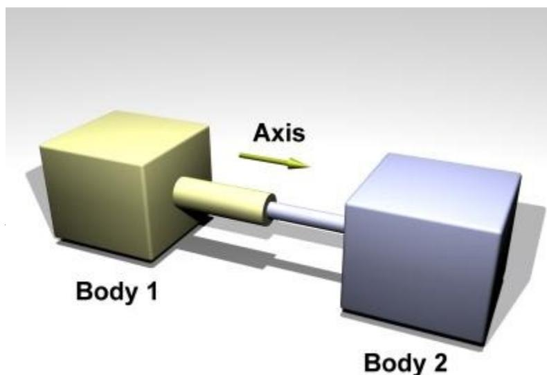
**Figure 11:** A Piston joint.
