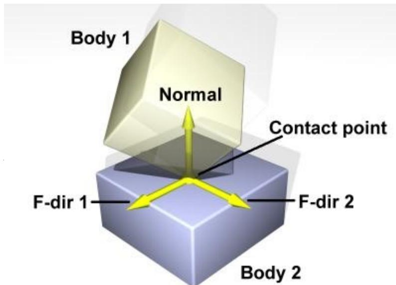
**Figure 10:** A contact joint.
