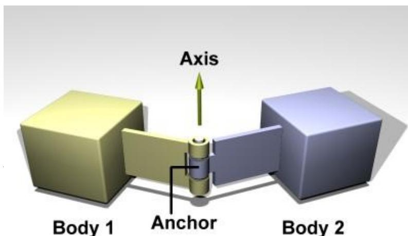
**Figure 5:** A hinge joint.
