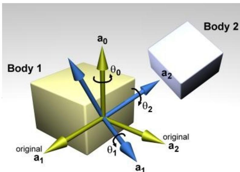
**Figure 11:** An AMotor joint with euler angles.
