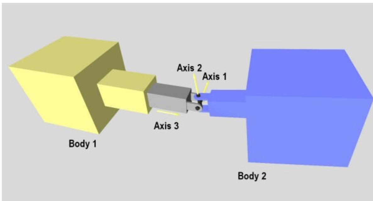
**Figure 10:** A Prismatic - Universal joint.
