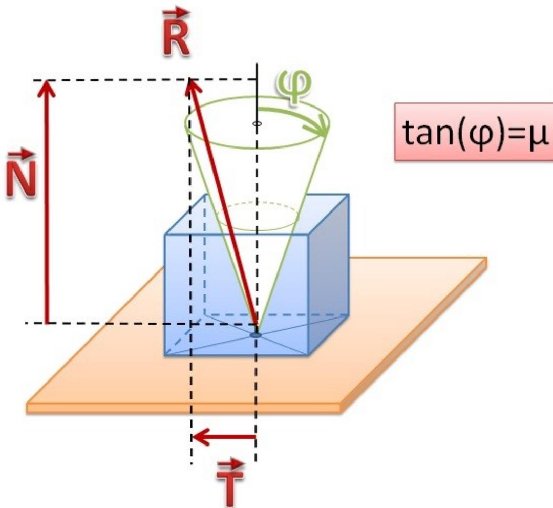
**Figure:** Angle of friction.
