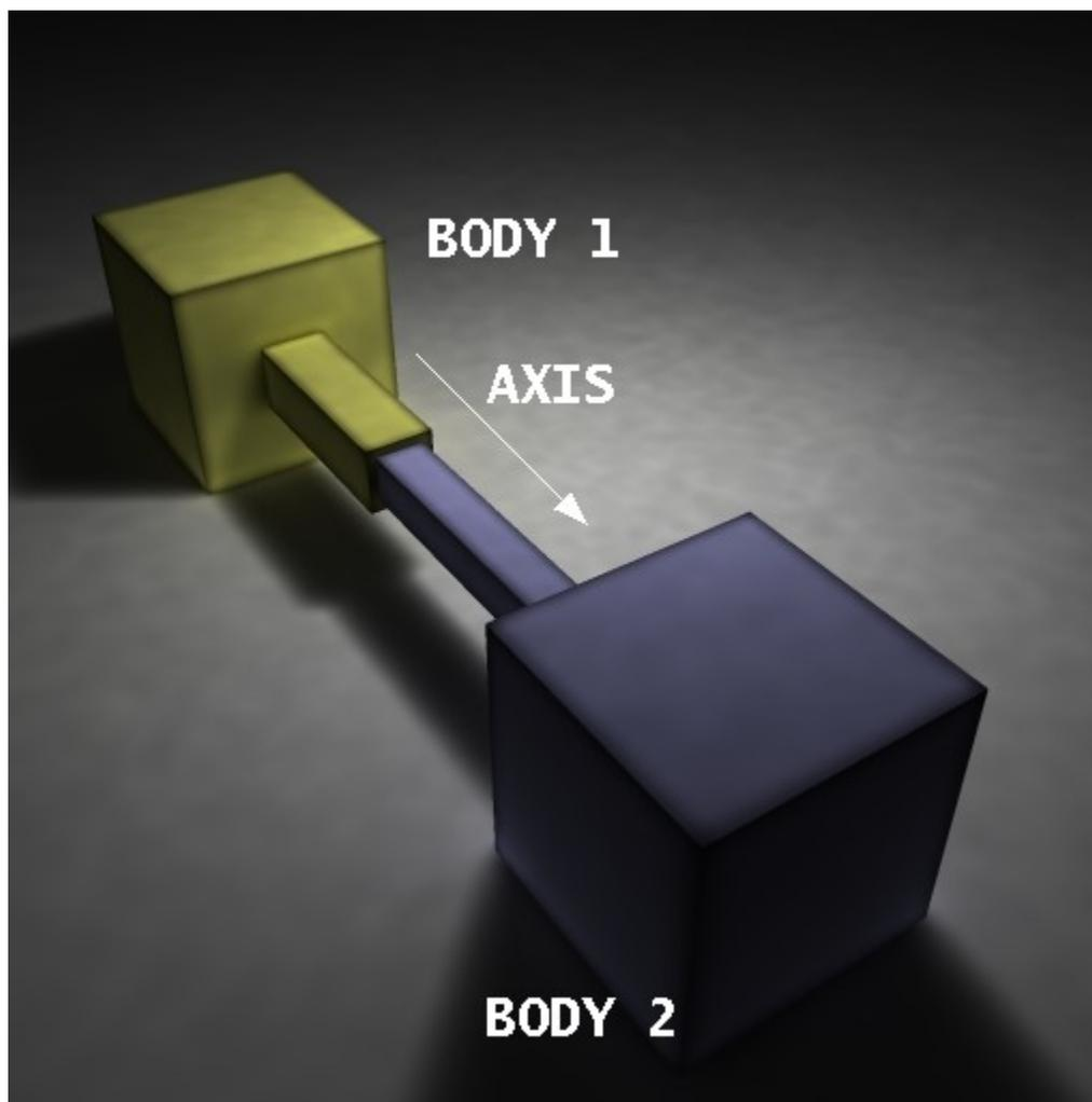
**Figure 6:** A slider joint.
