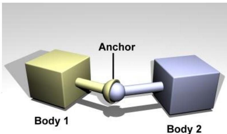
**Figure 4:** A ball and socket joint.
