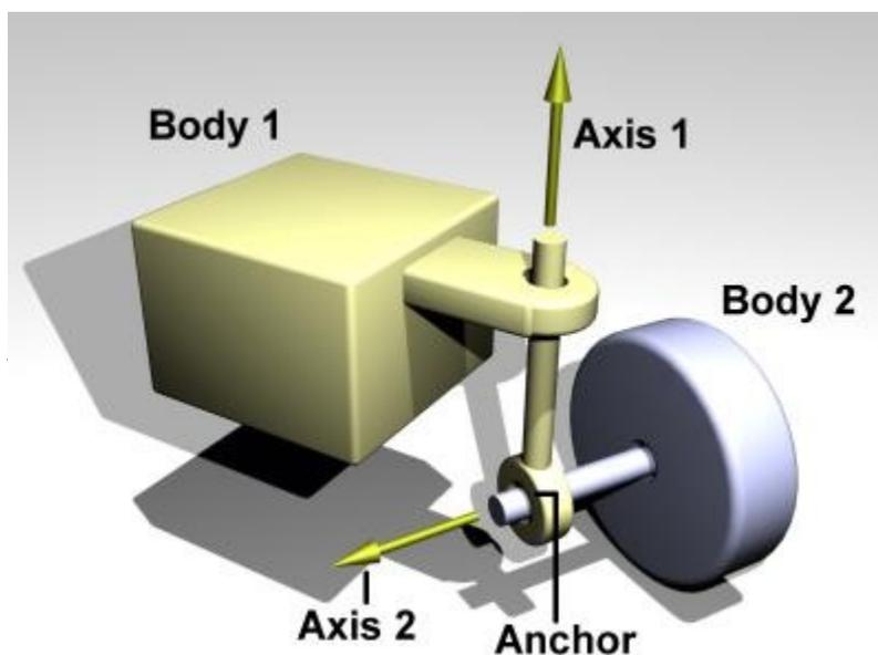
**Figure 8:** A hinge-2 joint.
